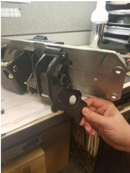
Step 2: Remove plate where Mcor is mounted
