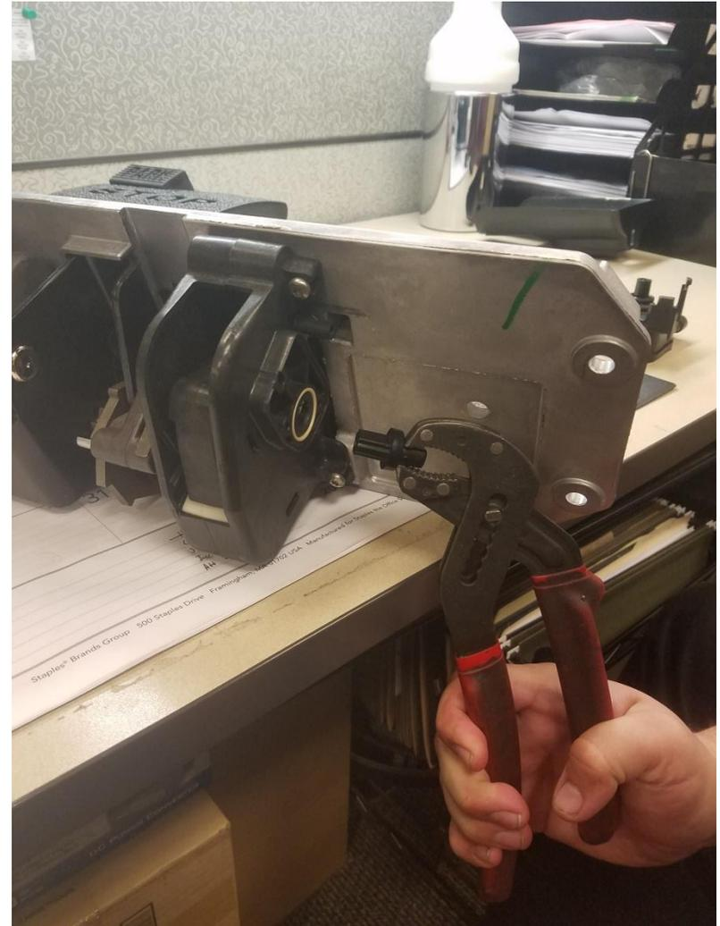
Step 4: Insert #8504 MCOR conversion kit and place screw back on
